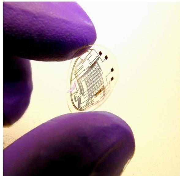
*Figure 1. A University of Washington researcher holds a contact with embedded metal interconnects.*
